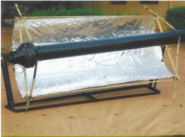
Plate 2: Parabolic trough solar collector with heater (absorber)
